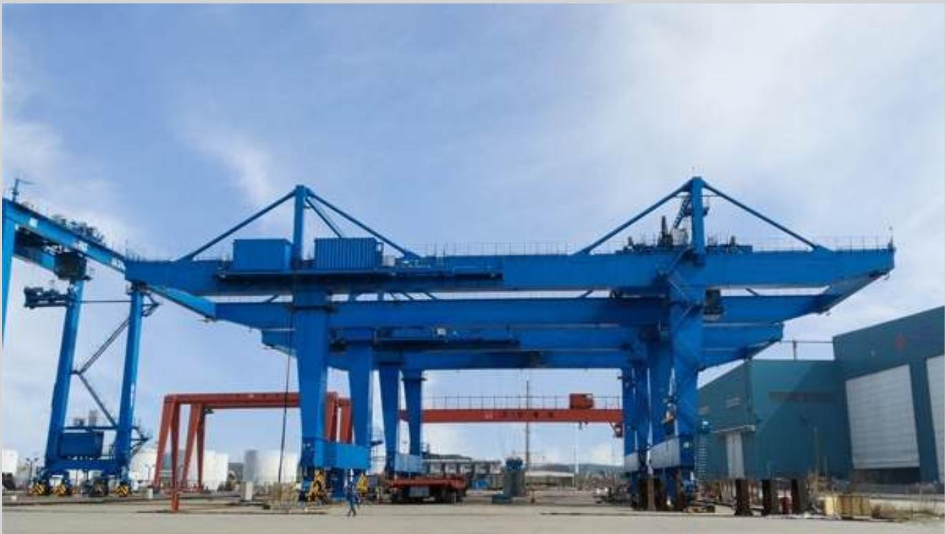
Rail-mounted gantry cranes (RMG) are manufactured to individual customer need in a variety of different stacking heights & spans, with 8 rope reaving, anti-sway & drive systems.
