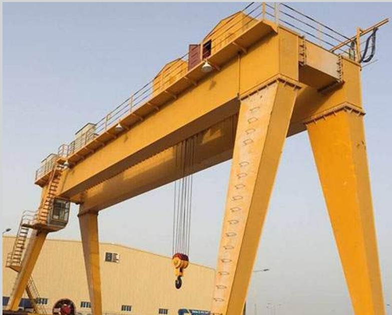
Goliath & Semi Goliath Cranes may be Single Girder or Double cranes, but they differ from E.O.T. Cranes, since they move on the rails fixed at ground level as compared to rails fixed at a height for E.O.T. cranes, these are in variable used for outdoor duty and is the most ideal material handling equipment to handle heavy loads in open yards
