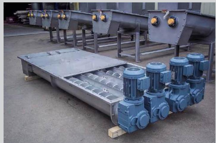
**EAGLE** makes screw conveying systems that are highly efficient in design. These systems are available in mild steel plates, hot-dip galvanized structures, and stainless steel structures. The screw conveying design is optimized to convey maximum raw material efficiently.
